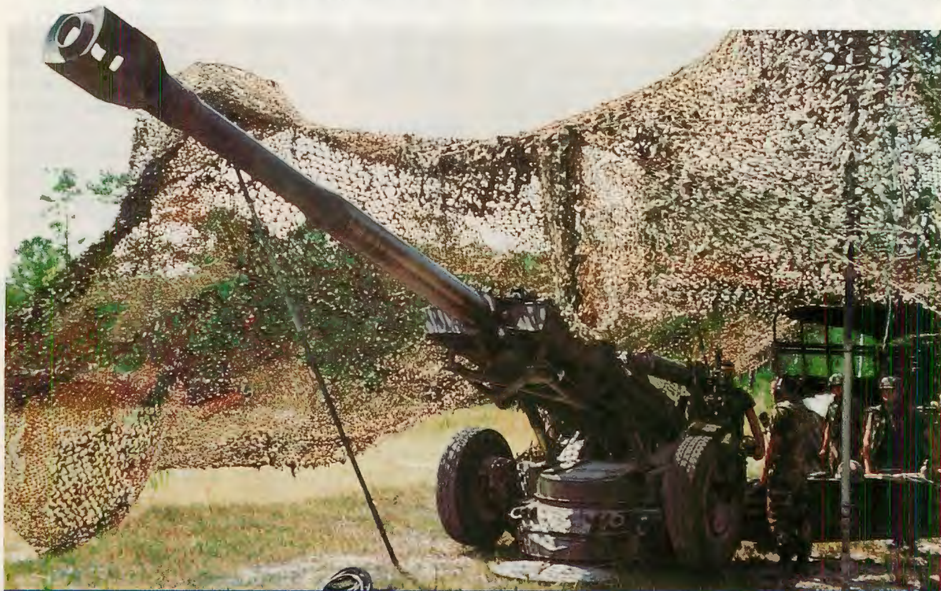
M198 155mm howitzer of Fox Battery, 10th Arty, 2nd Marine Division, awaits a fire order. Since World War I more wartime casualties have been caused by artillery fire than any other means. Photo: Douglas Burnham
